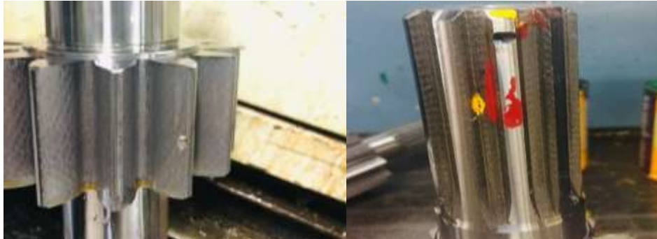
Figure- 1 Dent & damage on a gear shaft
